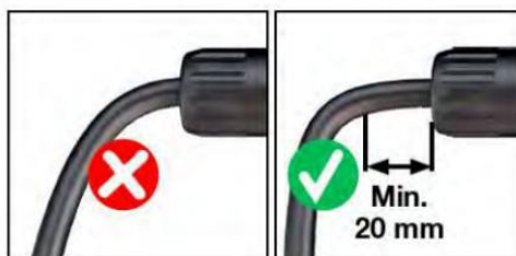
Figure 5-8 Cable routing
