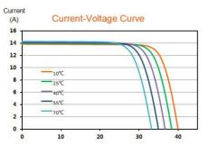
NMOT(Nominal Module Operating Temperature): Irradiance 800W/m Ambient Temperature 20°C, Wind Speed 1m/s **TEMPERATURE CHARACTERISTICS**
